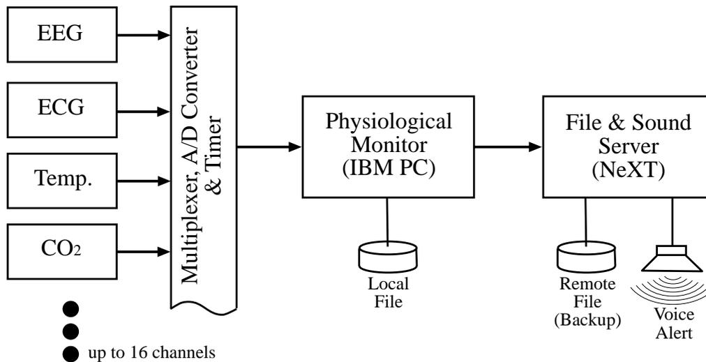
**Fig. 1** A block diagram is shown for the physiological monitoring system we employ (see text for details).
